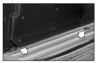
Your vehicle also has four cargo-area floor drains located under the cargo mat near the sides of the cargo area. These drains should be cleaned periodically to allow water to exit the cargo area.
